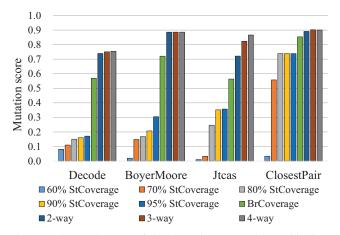
Fig. 11: Comparison on fault detection rate when achieving different *k*-way testing for BCT and techniques guided by statement or branch coverage
